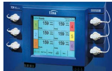
THE RADIOMETER TCM™400 IS USED TO MEASURE TISSUE OXYGEN TENSION.
